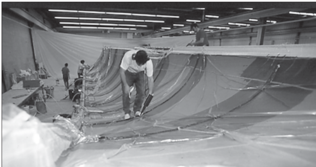
A large part of being vacuum bagged for resin infusion.
