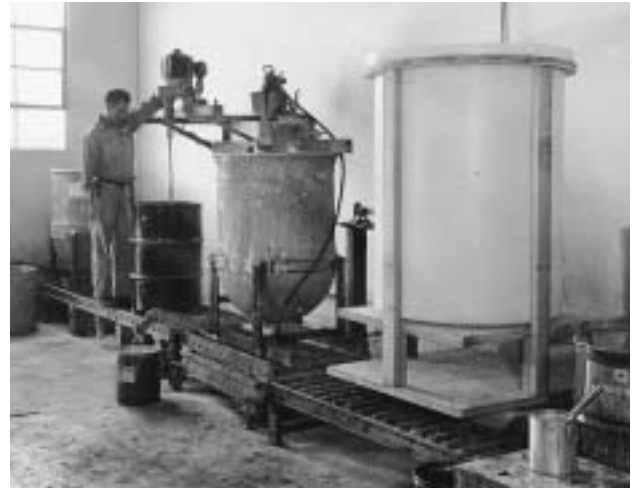
Resin-mixer Ike Dominguez, circa mid-60s. The Gill Company pre-impregnates it's own fabric.
